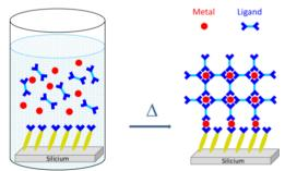
The systems under investigation are Fe-based MOFs obtained from Fe<sup>3+</sup> and carboxylate ligands (BDC, BTC...). The structural properties of the MOFs will be presented on the base of SEM, XRD and AFM characterizations.
