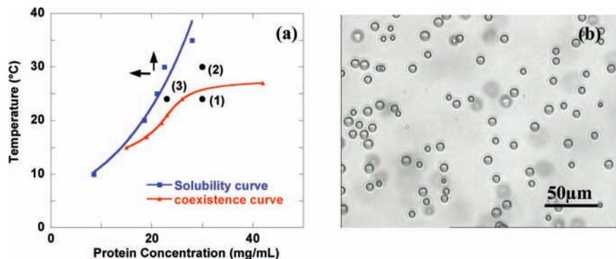
**Figure 6.** (a) Phase diagram of BPTI at pH 4.9 in 350 mM KSCN in the concentration range 0–50 mg/mL (after refs 12 and 32); and (b) observation by optical microscopy of the nucleation of droplets of the protein-rich phase in a supersaturated solution of BPTI (30 mg/mL) when temperature is decreased to 25 °C (point (1)).
