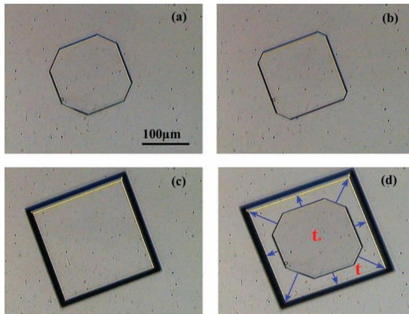
**Figure 2.** Growth of a BPTI crystal in 350 mM KSCN at pH = 4.9 across the trajectory shown in Figure 1. Panels a–c are frames of a time sequence obtained at different temperatures showing the evolution of the growth form as illustrated in (d), in which arrows indicate the face displacement with time.
