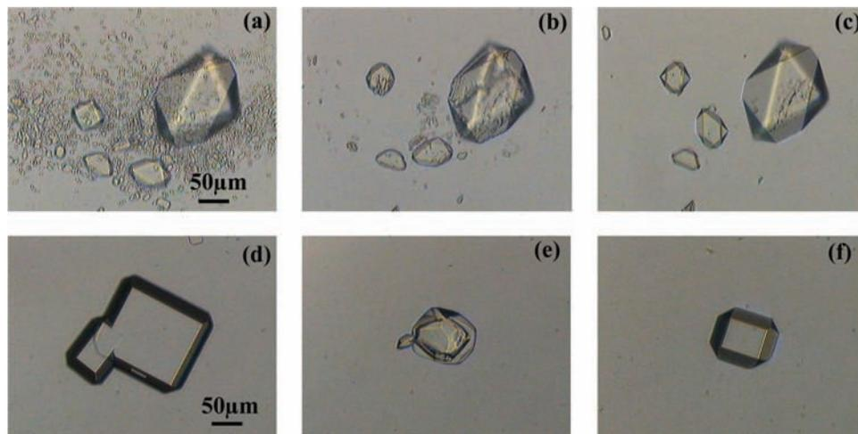
**Figure 4.** Kinetic ripening of B polymorph of  $\alpha$ -amylase crystals shown in (a), by (b) partial dissolution and (c) regrowth. Elimination of a macrodefect observed in (d) by (e) dissolution and (f) growth.
