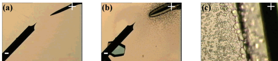
Figure 6. In situ observations under optical microscopy of lysozyme crystallization at 20 °C (lysozyme 25 mg/mL in 0.7 M of NaCl and 50 mM of sodium acetate buffer solution at pH 4.5) with a direct voltage of 0.9 V (experiment 2), at times of (a) 0 and (b) 12 h, and (c) a zoom of the layer formed at the anode. As reference, the W-electrode wire diameter is 125 \mu\text{m} (the + sign indicates the anode).
