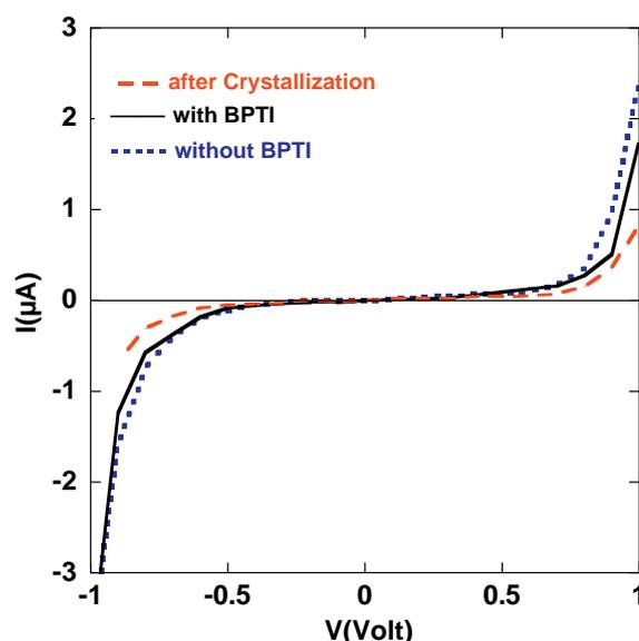
**Fig. 10.** Different  $I$ – $V$  curves for NaCl 1.6 M solutions at pH 4.5, without BPTI, 20 mg/mL and after crystallization.
