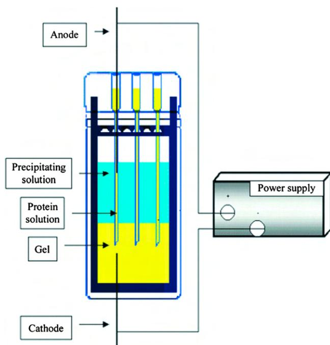
Fig. 4. Modified gel-acupuncture set-up of Mirkin et al. (2003), with permission of Acta Cryst. Wiley.
