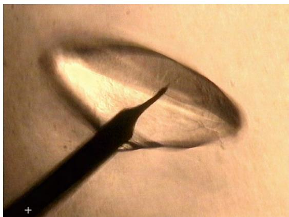
**Fig. 9.** BPTI (20 mg/mL – NaCl 1.6 M) nucleation in the vicinity of the tip in 0.5% agarose gel (0.8 V – 0.74  $\mu\text{A}$ ). As reference the W-electrode wire diameter is 125  $\mu\text{m}$  (+indicates the anode), (Hammadi et al., 2009) with permission of Crystal Growth and Design. American Chemical Society.
