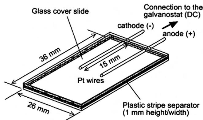
Fig. 5. Experimental set-up of the crystallization cell with parallel electrodes, 0.2 mm diameter (Moreno and Sasaki, 2004), with permission of J. of Crystal Growth. Elsevier.
