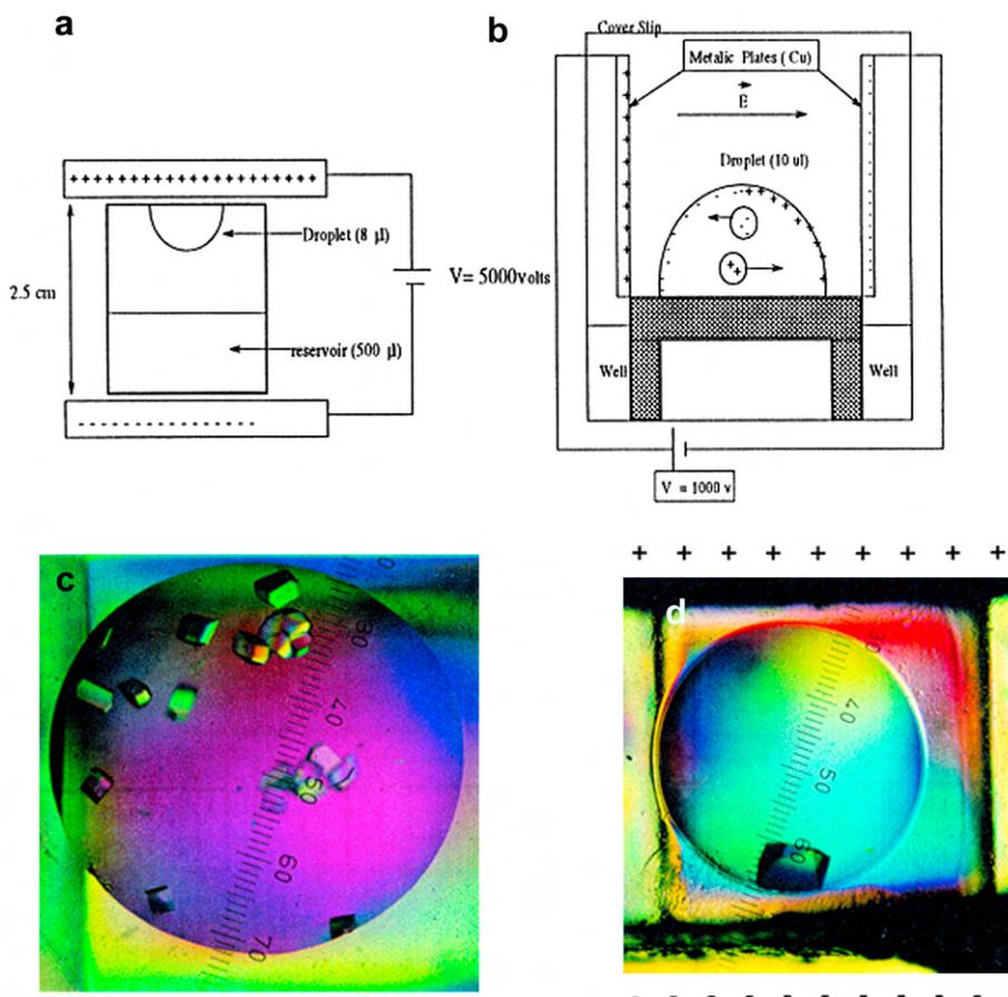
**Fig. 2.** The two crystallization devices developed by Taleb et al. (1999): (a) the whole Linbro plate is placed between two metal plates connected to a power supply, (b) the droplet is directly placed between two metal plates connected to a power supply; crystals form in the drop: (c) without electric field and (d) under electric field, with permission of J. of Crystal Growth. Elsevier.
