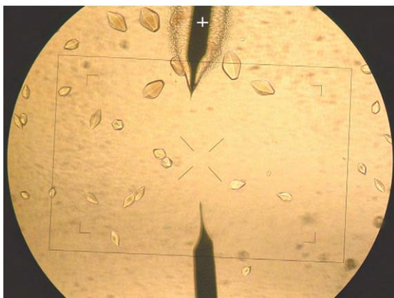
**Fig. 8.** In-situ observations under optical microscopy of BPTI crystallization at 20 °C with direct voltage of 0.785 V at  $t = 18$  h as reference the W-electrode wire diameter is 125  $\mu\text{m}$  (+indicates the anode).
