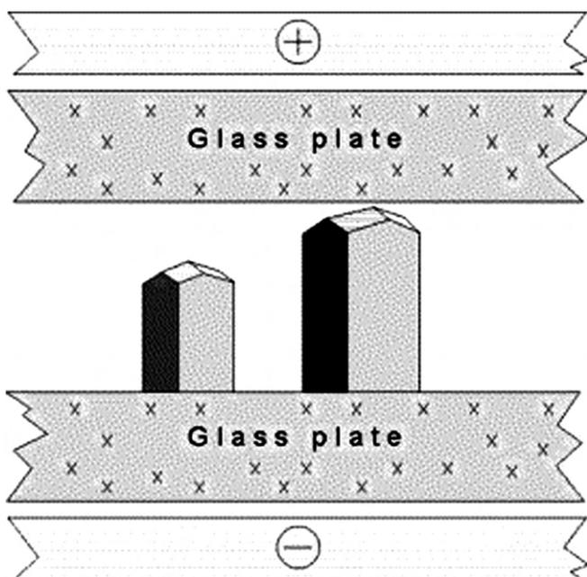
**Fig. 3.** Schematic representation of the growth cell of Nanev and Penkova (2002), together with the two electrodes and two HEWL crystals oriented along c-axis, with permission of Colloids and Surfaces A: Physicochemical and Engineering Aspects. Elsevier.
