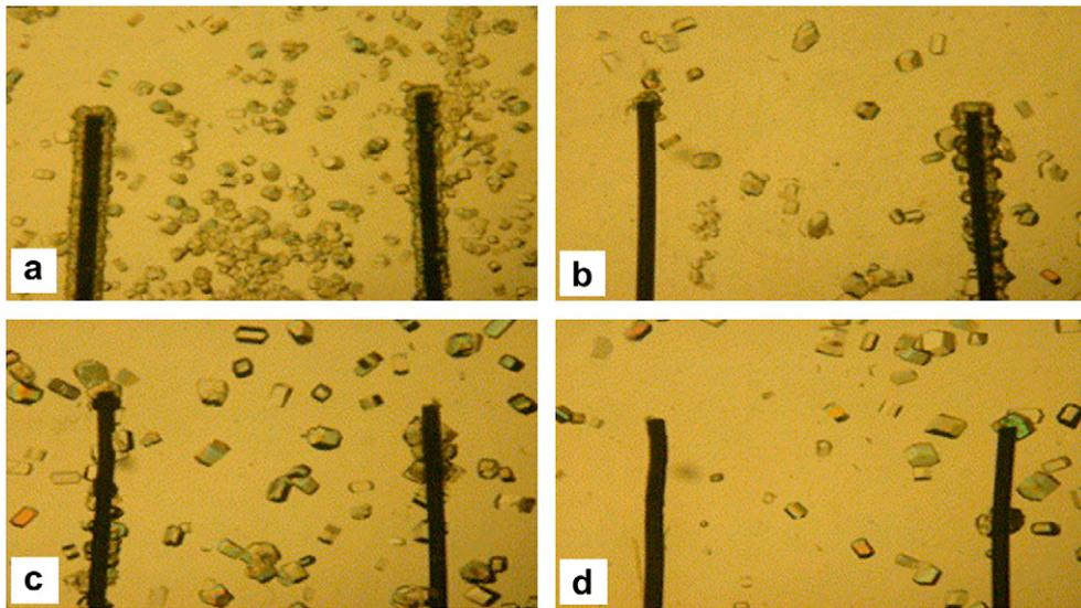
**Fig. 6.** Images from (Moreno and Sazaki, 2004), (a) Corresponds to the experiment in solution without current, (b) with current, (c) growth in gels without current, and (d) growth in gels in the presence of a constant current, with permission of J. of Crystal Growth. Elsevier.
