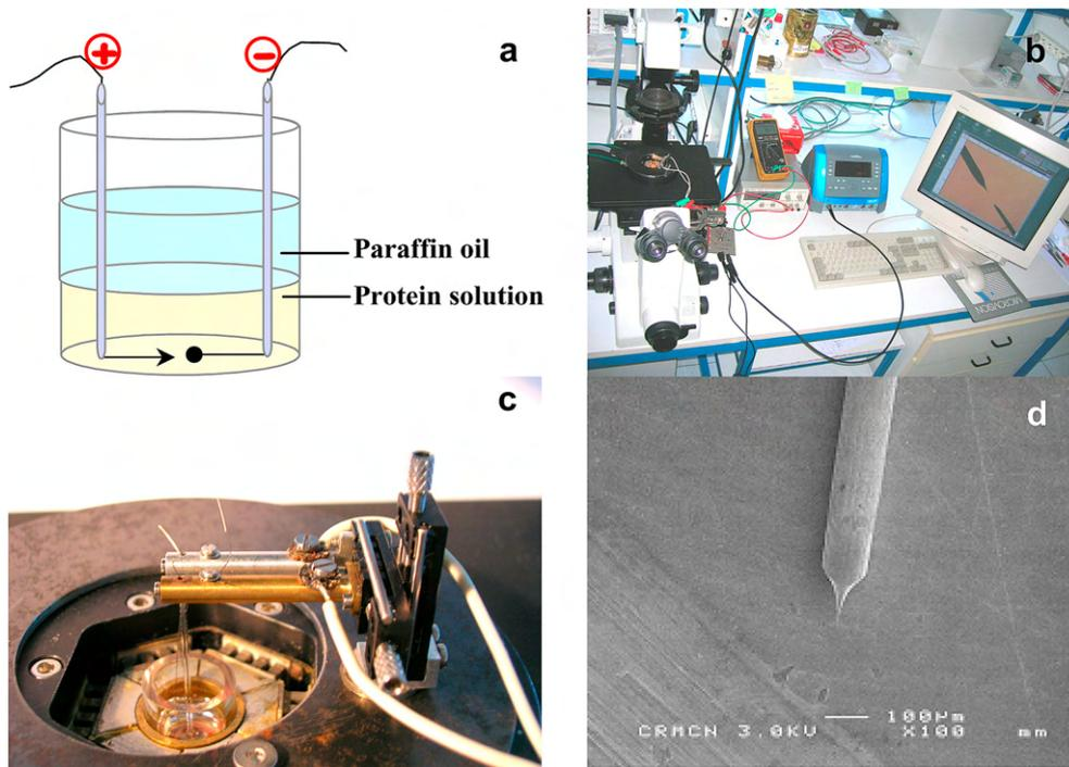
**Fig. 7.** (a) Crystallization cell with the 2 electrodes, (b) whole experimental set-up, (c) Y,Z positioning stage for the electrodes and (d) sharp tip of the electrode (Hammadi et al., 2007) with permission of Crystal Growth and Design. American Chemical Society.
