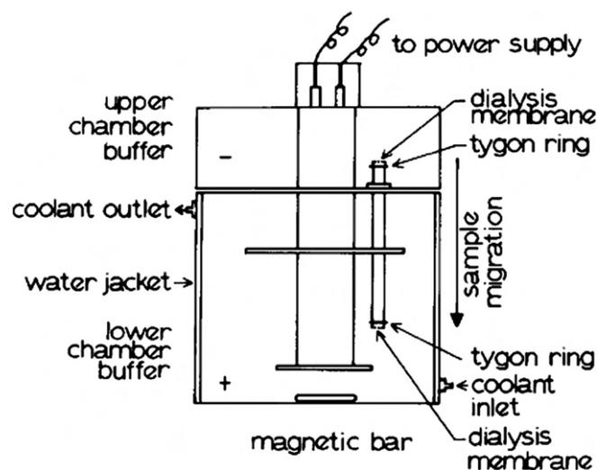
Fig. 1. Electrophoresis diffusion set-up of Chin et al. (1976), with permission of J. Biol. Chem.
