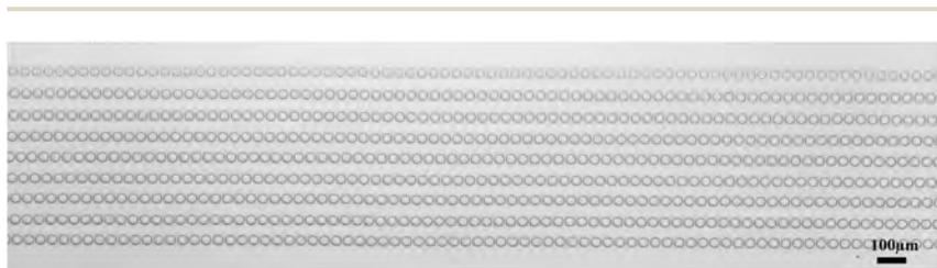
Fig. 2 Array of droplets ( $\sim 720$ ) of NaCl solutions generated through the layer of inert DMS oil.
