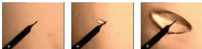
**Figure 3.** BPTI (20 mg/mL - NaCl 1.6M) nucleation in the vicinity of the tip in 0.5% agarose gel (0.8 V - 0.74  $\mu\text{A}$ ), length of experiment 12 h. As reference, the W-electrode wire diameter is 125  $\mu\text{m}$ .
