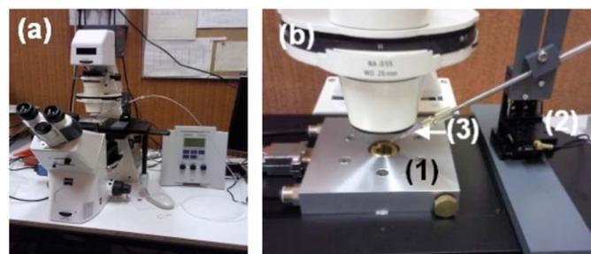
**Fig. 1.** (a) Image of the whole experimental set-up and (b) zoom of the previous image: (1) thermostatted crystallization-well, (2) XYZ miniature translation stages and (3) glass capillary.
