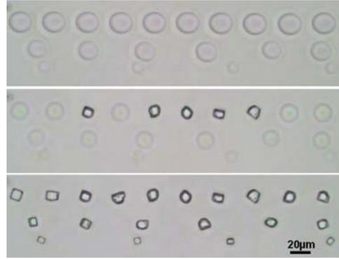
FIG. 2 (color online). Time sequence showing nucleation and fast growth of NaCl crystals. (a) At  $t = 0.45$  s 4.5 M NaCl microdroplets of volumes ranging from 3 to 1 pL are generated (assuming a spherical shape for the droplet), (b)  $t = 4638$  s, and (c)  $t = 6120$  s. All the micrographs are at the same magnification.
