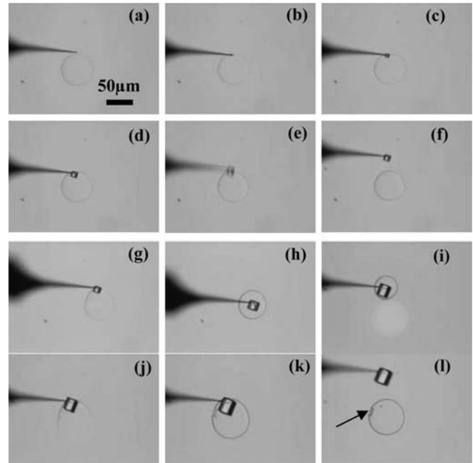
FIG. 4. Panels (a)–(l) represent a time sequence showing the nucleation and growth of NaCl at supersaturation  $\beta > 1.97$ . (a) 0.7 M NaCl initial droplet size  $56 \mu\text{m}$  ( $\approx 51 \text{ pL}$  assuming a spherical shape for the droplet). All the micrographs are at the same magnification. See Supplemental Material [17] for a movie of this process.
