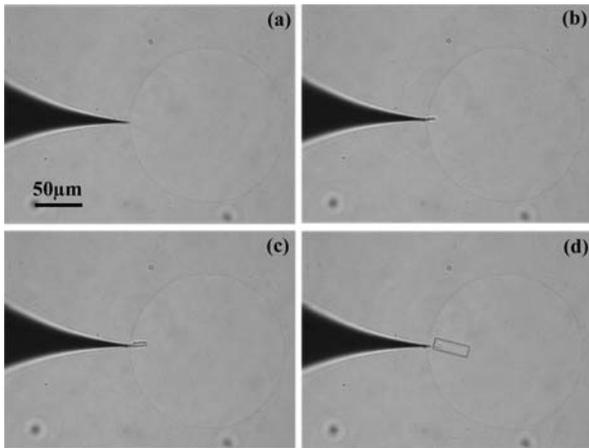
FIG. 3. Panels (a)–(d) represent a time sequence showing the nucleation and growth of KCl in DMS oil, initial condition: undersaturated KCl solution ( $\beta = 0.5$ ), (a) droplet size  $147 \mu\text{m}$  ( $\approx 1.66 \text{ nL}$  assuming a spherical shape for the droplet). All the micrographs are at the same magnification, the time between (b) and (d) is 1.3 s.
