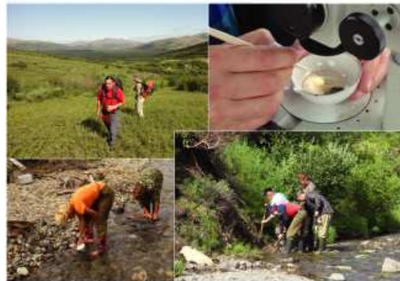
Figure 15. Field operations at the Listvenitovy stream (clockwise): mapping the structural geology, examining mineral samples, extracting clay from areas along the stream, and panning the clay down to mineral separates.
