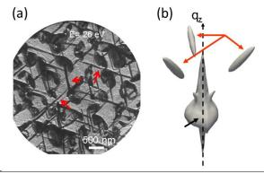
Fig. (a) Low Energy Electron Microscopy image of the surface of GeTe thin film grown on Si(111). (b) Corresponding 3D reciprocal space map around GeTe  $(222)_c$  (iso-intensity surface) for a 60 nm-thick film).
