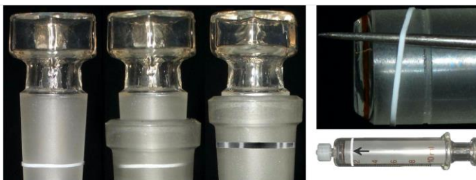
Figure 1. Figure caption. Left: PTFE-sealing ring fixed elastic (no groove necessary). Middle: Sealing ring intransparent without pressure. Right: Sealing ring transparent under sealing pressure. Far right: A similar PTFE ring and a piston groove make an all-glass-syringe gastight.
